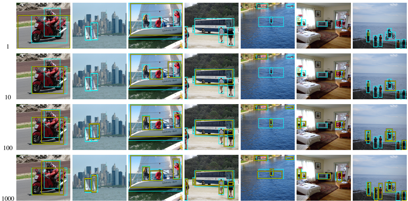
Fig. 16: Qualitative results for increasing number of windows. We show the accuracy of the objectness measure as a function of the number of windows it returns. Each row shows the results obtained when sampling 1, 10, 100, and 1000 windows. We mark in yellow windows correctly covering a ground-truth object (cyan); if there is more than one correct window, the most overlapping one is shown. As we sample more windows, more objects are detected and the accuracy of the windows covering them continuously increases. Sampling 1000 windows covers nearly all objects with high accuracy. Notice that 1000 is several orders of magnitude smaller than the number of all windows in the image.
