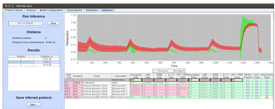
Fig. 2. Example parameter inference of a defined protocol, the parameter values in red are inferred from observed experimental data. The graph shows a sample simulation using these parameter values compared against the supplied experimental data.
