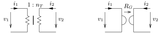
Figure 2: Left: Transformer, of turns ratio n_T . Right: Gyrator, of gyration constant R_G .
