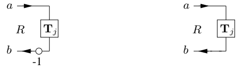
Figure 3: Left: MDWD inductor, of direction t_j and port resistance R = 2L/T_j . Right: MDWD capacitor, of direction t_j and port resistance R = T_j/2C .
