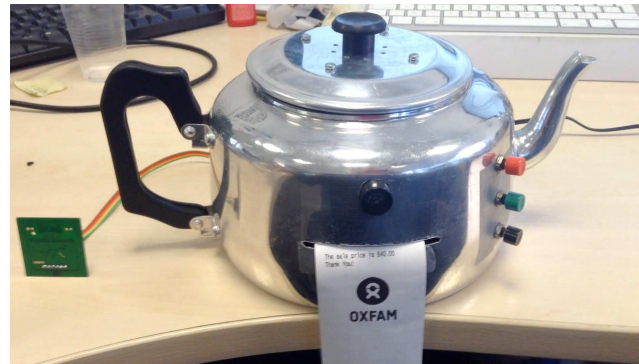
Figure 2. Version 3 of the Hagggle-O-Tron with thermal printer, RFID reader, speaker holes on top and buttons to support price negotiation.
