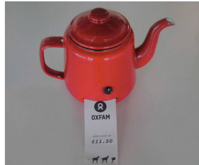
Figure 1. Version 1 of the Haggle-O-Tron with thermal printer, microphone / speaker grill (on side) and camera peephole to support engagement with shopper.
