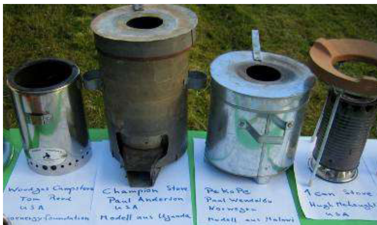
Figure 3: Four micro-gasification stoves reviewed by GIZ, source: [11]
