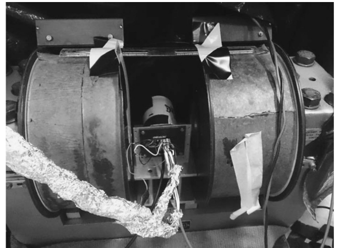
Fig. 4. Setup with small MaPMT enclosure mounted between pole shoes of stronger magnet.
