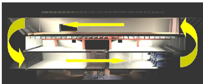
Figure 5 Wind tunnel vertical section
