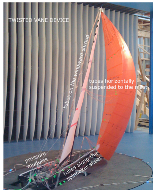
Figure 1: the AC33 1/15 th scale model set up for tests.
