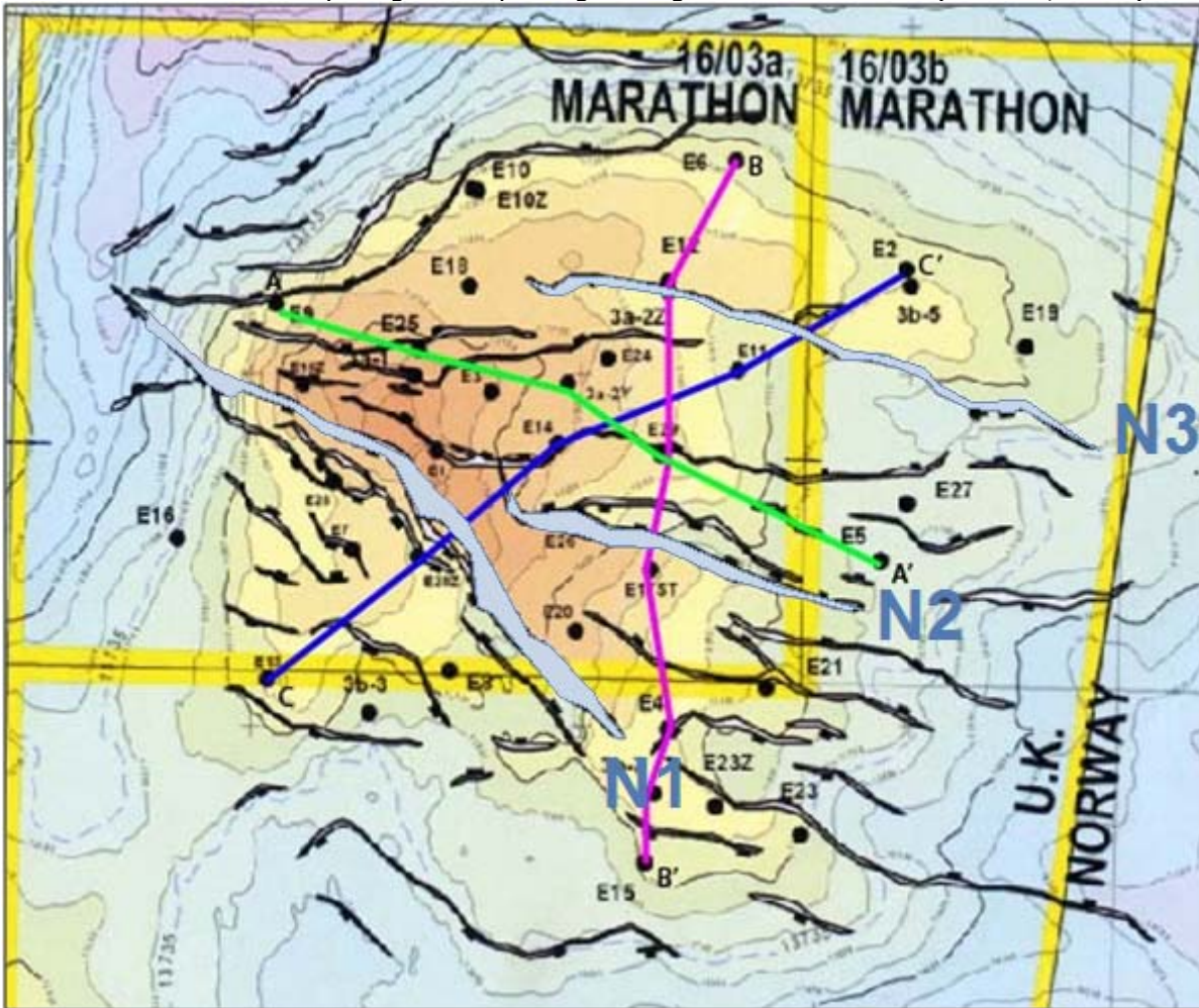
Figure 86 Map view illustrating three correlation transects: A-A' (green), B-B' (purple), C-C' (blue) across the Brae Formation. Note the presence of the ESE - WNW trending faults, major faults N1 – N3 (grey) are also shown.
