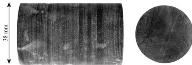
Figure 39 Image of the 38mm diameter core non fractured caprock sample, B-c from the North Sea Brae field.
