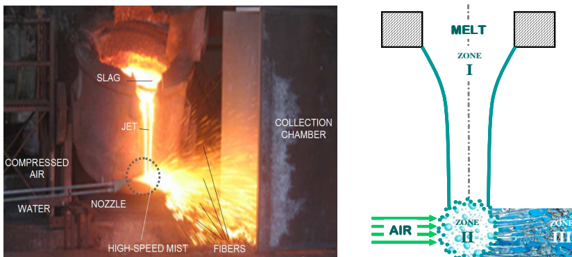
Figure 2. (a) Molten slag fiberization demonstration unit, (b) Mathematical modeling strategy and zone definition.
