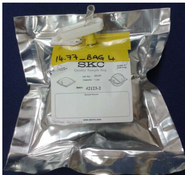
Figure 1 Foil bag (FlexFoil PLUS, SKC Inc.) showing adapted connection for sample collection.
