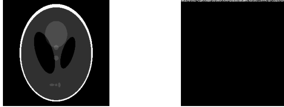
Figure 3: An example of a piecewise constant image: the 256 \times 256 Shepp Logan phantom (left); and an image with the same cosparsity, \ell = 128014 , but whose cosupport is associated with an empirically maximum subspace dimension (right).
