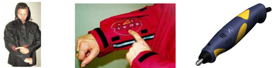
Making fabrics and surfaces touch sensitive: - An interface for an MP3 player in the sleeve of a jacket and a power-drill 'easy-grip' variable speed control
