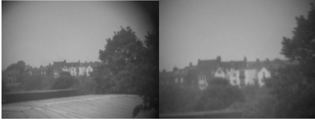
Fig. 8. Zoom-switching. The image on the left corresponds to a magnification factor of \times 0.81 , the right of \times 1.24
