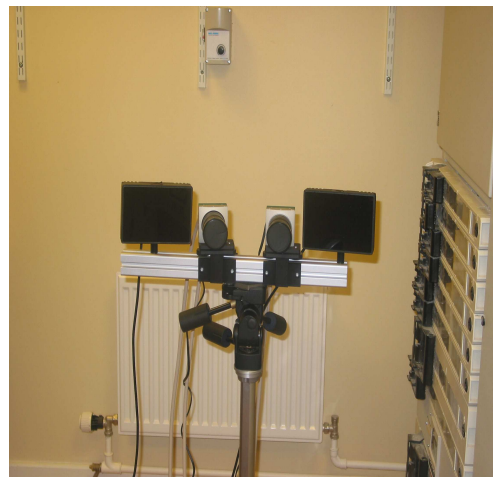
Fig. 1. Stereo rig of the high-speed scanner
