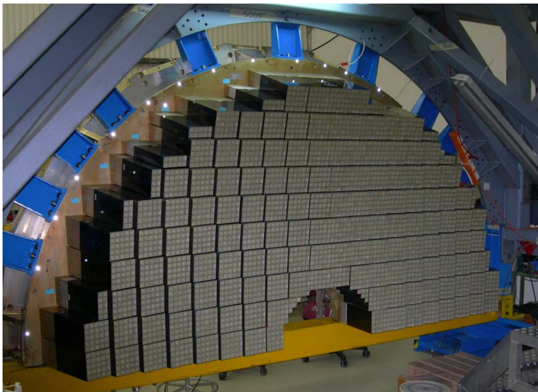
Figure 4.7: An endcap Dee, fully equipped with supercrystals.
