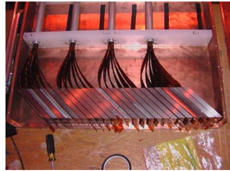
Figure 6.5: Photograph of the ZDC HAD section.
