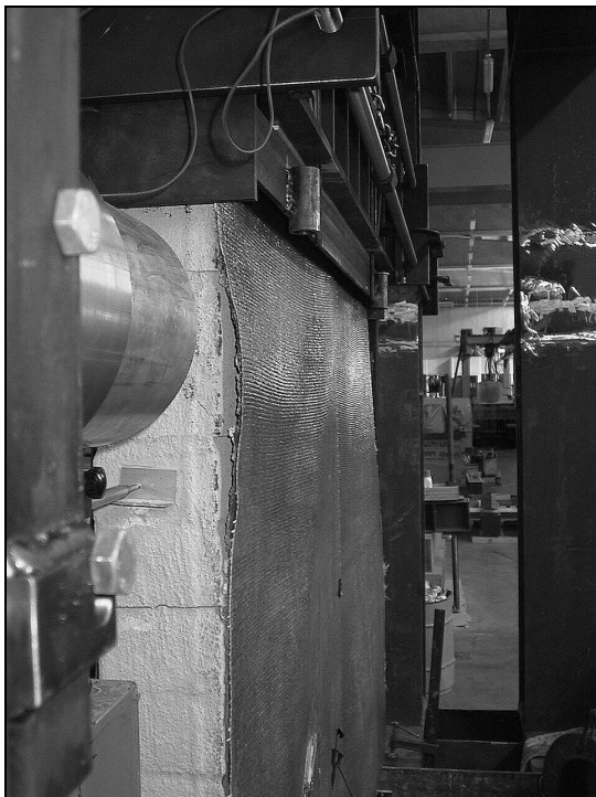
Figure 10 – De-bonding at loading point (concrete 2)
