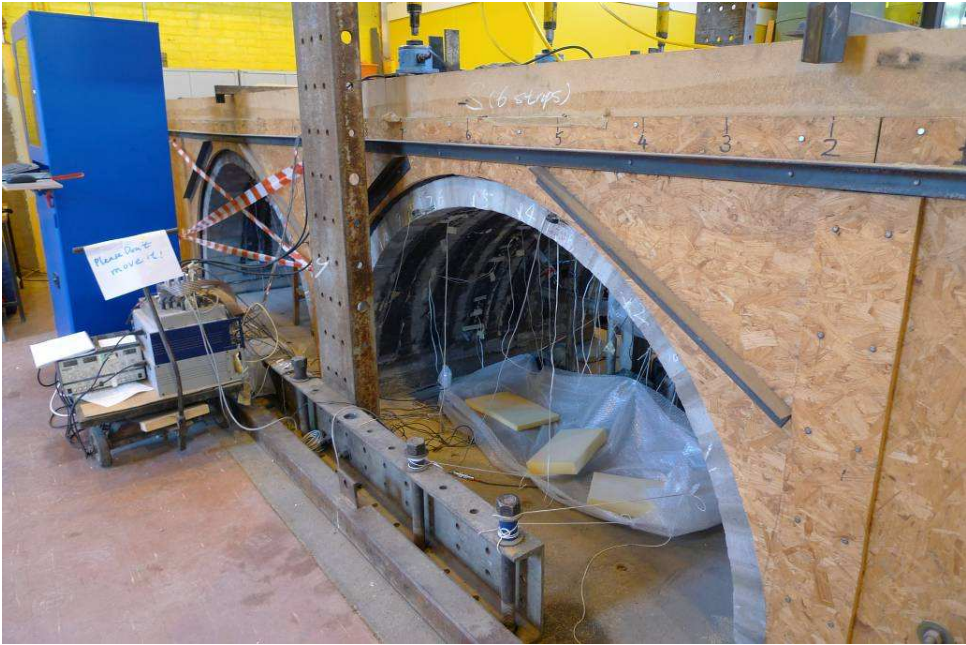
Figure 2. The western elevation of the arches after repair with CFRP
