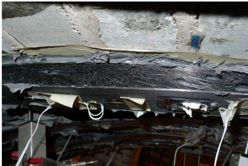
Figure 9. Debonding of the CFRP plate within the laminate, plate Ps 4
