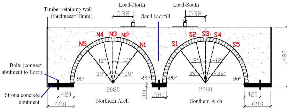
Figure 1: Schematic arch model (dimensions in mm)
