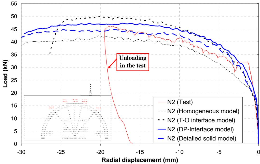
Figure 5: Comparison between FE predictions and experiment
