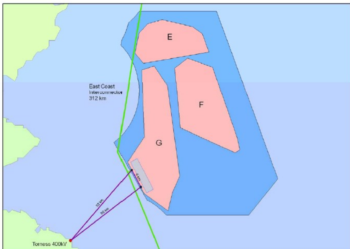
Fig. 4. Firth of Forth zone connection overview. The figure shows the two potential connection routes to the 400Kv substation at Torness. Polygon E represents Phase 1 of development and connection, followed by G (Phase 2) and then F (Phase 3). Source: The National Grid and Crown Estate (2009:44)
