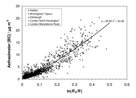
Figure 3: Linear fit to BC vs  $BSI_{BRITISH}$  for  $BSI_{BRITISH}$  <15  $\mu g$  m<sup>-3</sup> at all sites.
