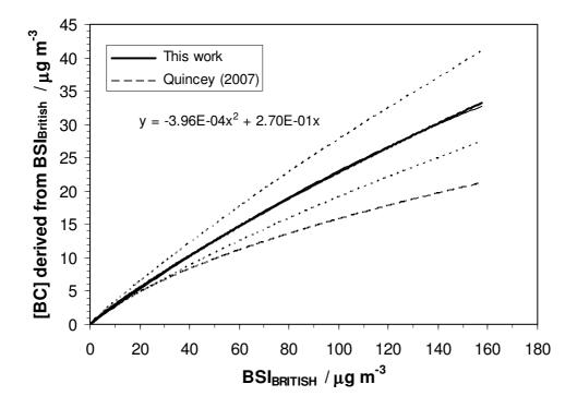
**Figure A1:** Reflectance values corresponding to values of BSI<sub>BRITISH</sub>, as per the British Standard 1747:2:1969 Black Smoke calibration. The best-fit quartic polynomial equation is shown.
