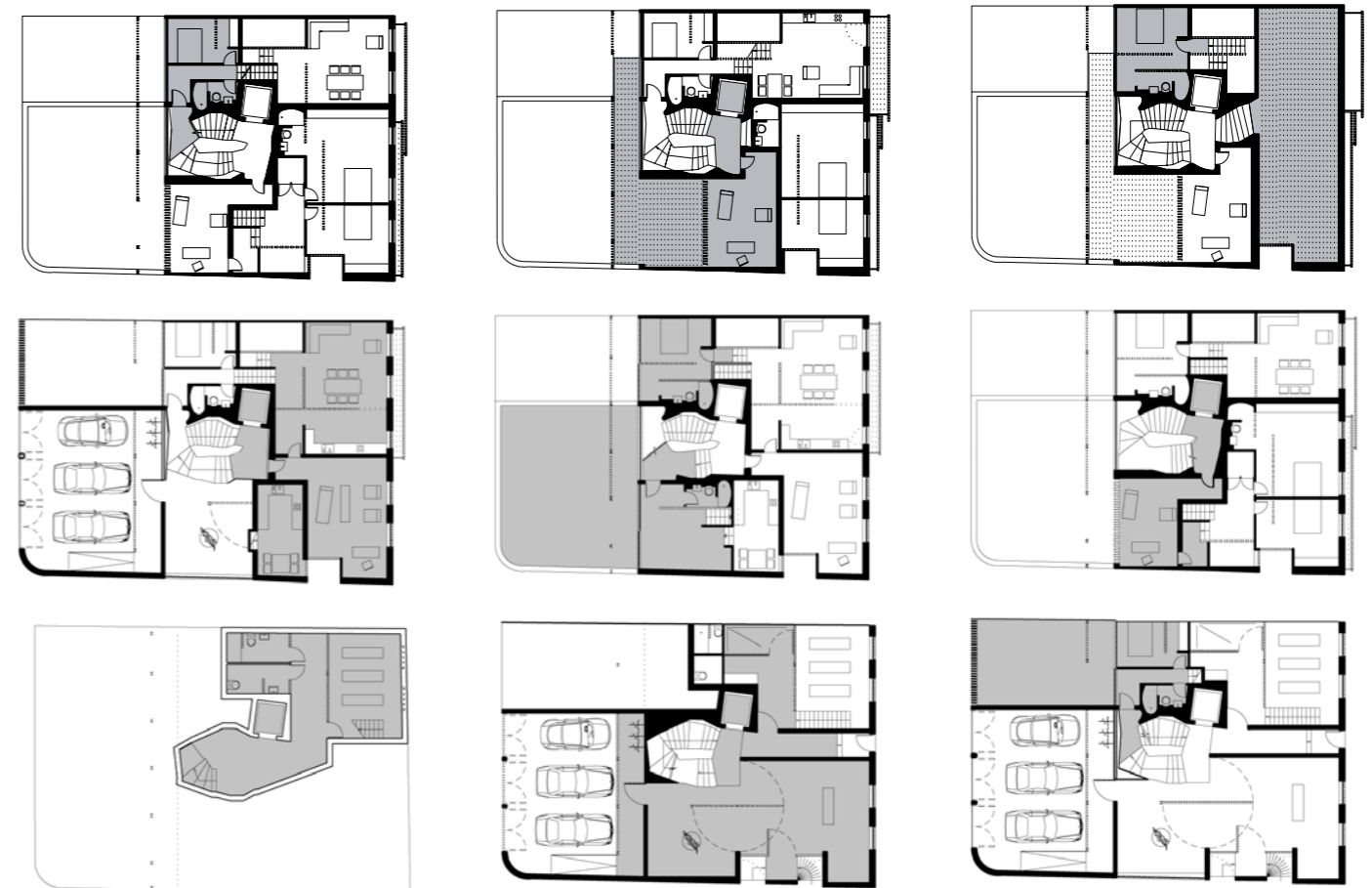
Plans showing stair rising (left-right, bottom-top) through series of half levels separating work and live programmes.
