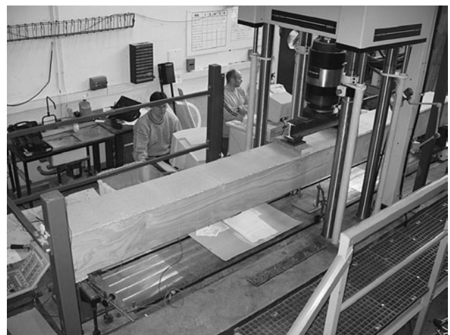
Figure 2. Test arrangement on a pair of 4.7 m span steel-timber joists under a central point load
