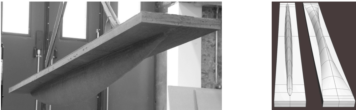
Figure 4 Form-active beams: left(a) Initial geometry, right (b) Initial and final geometry
