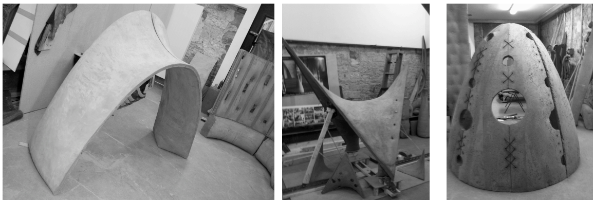
Figure 5 Shell using fabric formwork from the left (a) Gaussian, (b) Hypar, (c) Dome
