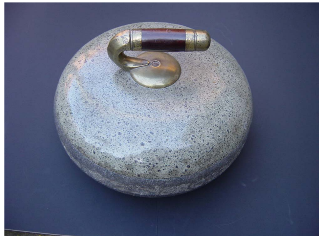
Figure 2. Photograph of a curling stone formed from Ailsa Craig Blue Hone (diameter 29 cm).
