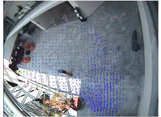
Figure 1: Eigenflows for the simulated normal training set (elements in the first eigenvector).
