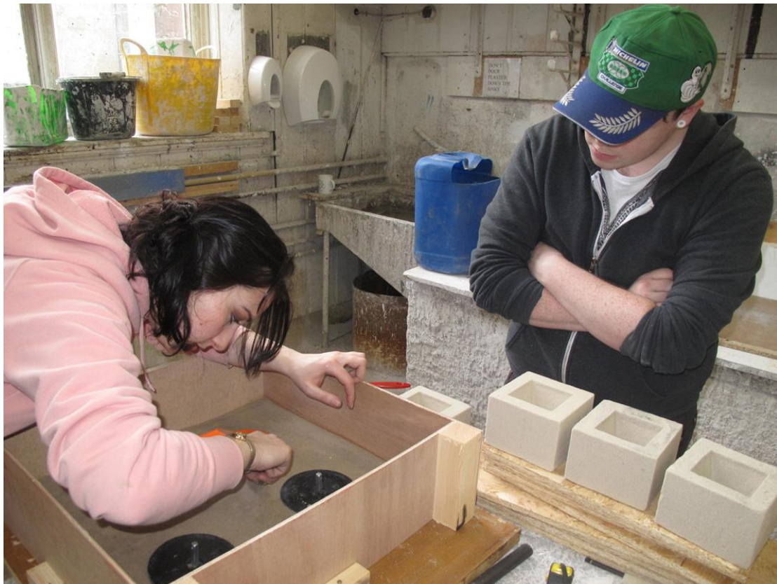
Resin bonded sand mould preparation with Edinburgh Sculpture Workshop casting technician Kate Ive during University of Edinburgh Innovative Learning Week 2012.
