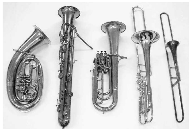
FIG. 3. Five brass instruments used in playing tests. From left to right: Kaiserbaryton, ophicleide, bass saxhorn, bass trombone, and tenor trombone.
