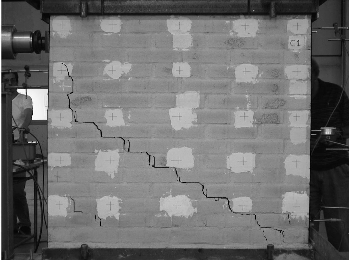
Figure 7 - Crack pattern in the unreinforced concrete panel (concrete 1).
