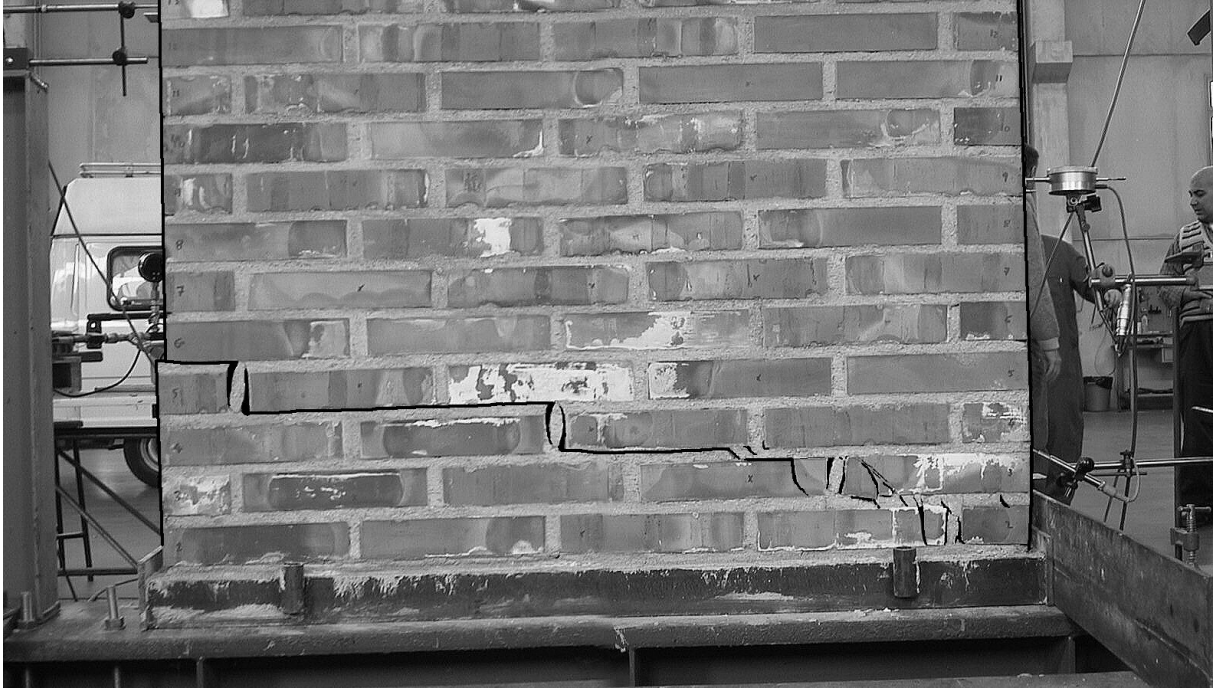
Figure 6 - Crack pattern in the unreinforced clay panel (clay 1).
