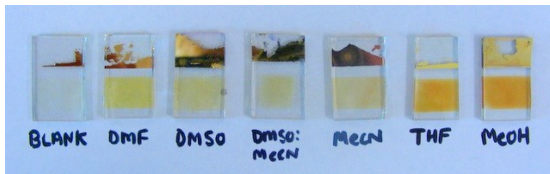
Figure 8. Sensitisation of \text{TiO}_2 slides by 3c left in various solvent dye baths for 48 h (unsensitised, DMF, DMSO, DMSO: \text{CH}_3\text{CN} (1:1), \text{CH}_3\text{CN} , THF and methanol respectively) . The nanocrystalline \text{TiO}_2 area is the rectangle in the lower portion the slide.
