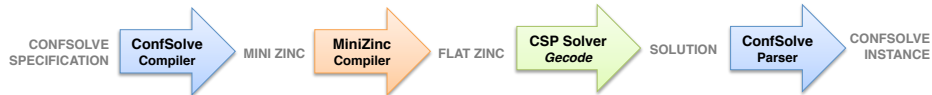
Figure 1. The architecture of ConfSolve. A ConfSolve instance is a structured text file representing a single solution.
