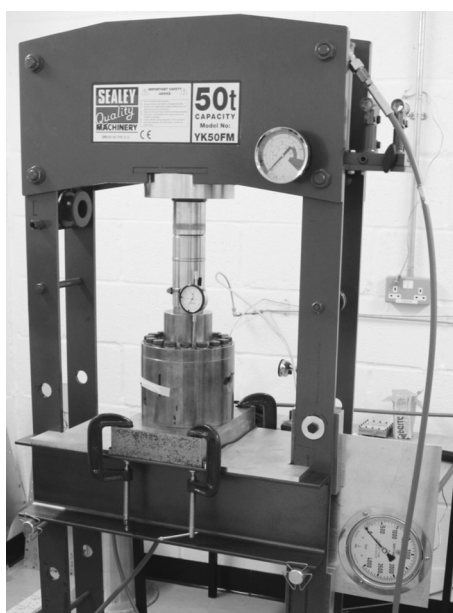
FIG. 5. Gas loader assembled in the hydraulic press. Visible are the pressure vessel, the dial gauge monitoring the piston position, and the pressure gauge showing pressure inside the vessel.
