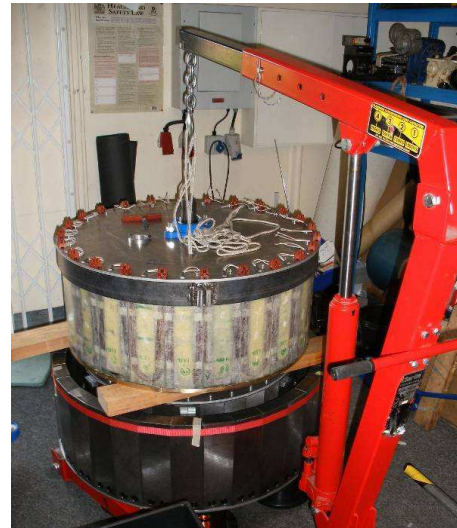
Figure 4: Assembly of stator and rotor with an engine hoist
