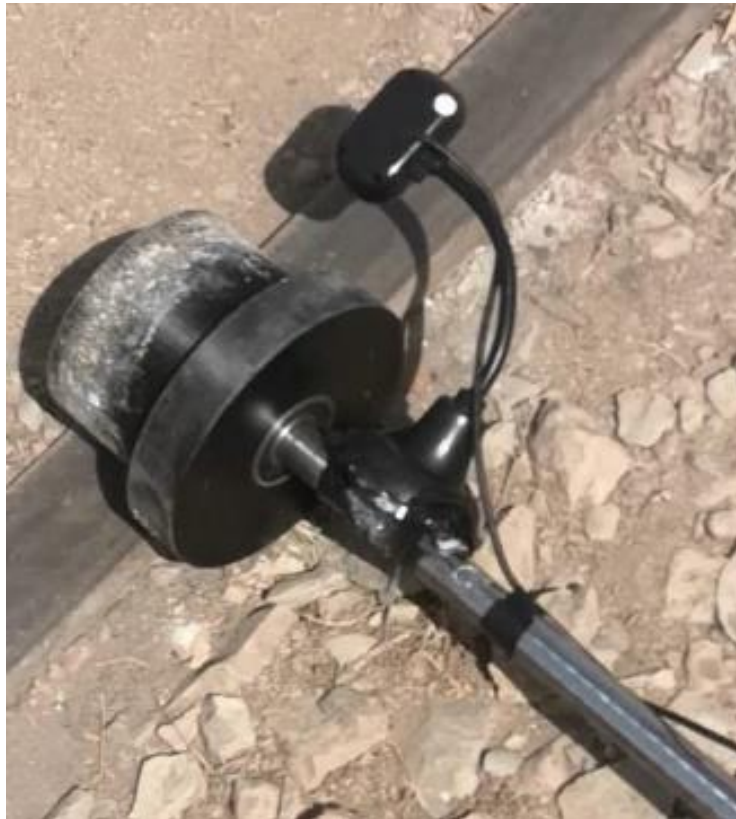
Figure 1. Camera Mounted on Track Recording Vehicle
