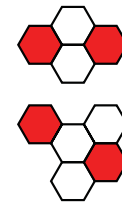
Fig. 6. A Surface configuration never contains the above patterns of empty space (white) and robotic subunits (red).
