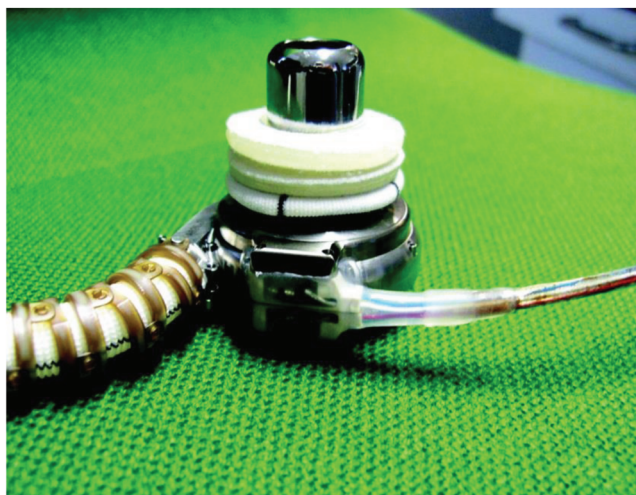
Figure 4. Reduction of the effective length of the inflow cannula with 2 dacron velour-covered 5-mm silicon suture rings. Copyright 2011, American Heart Association, Inc.; reproduced with permission from Figure 3 of Krabatsch et al. 47
