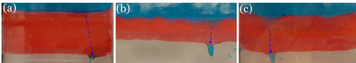
Figure 5. Elastic instability prior to the leak. (a) For a seal of low precompression ( \varepsilon = 10\% , l/h = 6.7 ), prior to the leak, the edge of the hydrogel is nearly straight. (b) For a seal of moderate precompression ( \varepsilon = 30\% ) and a relatively small aspect ratio ( l/h = 2.2 ), prior to the leak, the straight edge of the hydrogel becomes unstable and forms a wavy shape. (c) For a seal of high precompression ( \varepsilon = 37\% ) and a relatively large aspect ratio ( l/h = 4.4 ), prior to the leak, the straight edge of the hydrogel becomes unstable but does not form a wavy shape.
