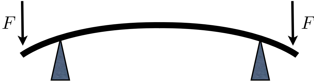
FIG. 3: (Color online) Edge torques acting on a membrane. The part of membrane that lies between the triangular supports, is influenced by external torques connected by a moment arm to the support. Torques are the consequence of external forces F acting on the sides of the membrane that lie outside the supports.
