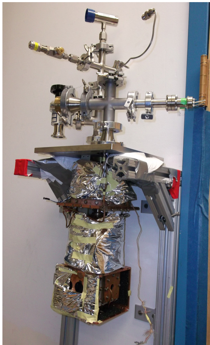
Figure 2.9: The experimental cell is mounted to the bottom of an IR labs dewar and cooled with liquid nitrogen and liquid helium. The cell nearly fills the entire 4 Kelvin region.
