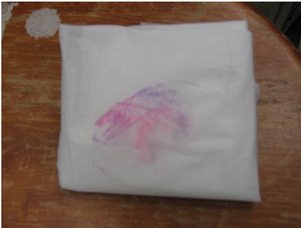
Figure 2.3: Nile Red residue on a chem wipe swab from the near the top of the 300K vacuum chamber in a region with no direct lines of sight to the molecule injection line. A thin coating of Nile Red on the entire 300 K vacuum chamber indicates that even molecules with very low vapor pressures can reach anywhere within the vacuum system.
