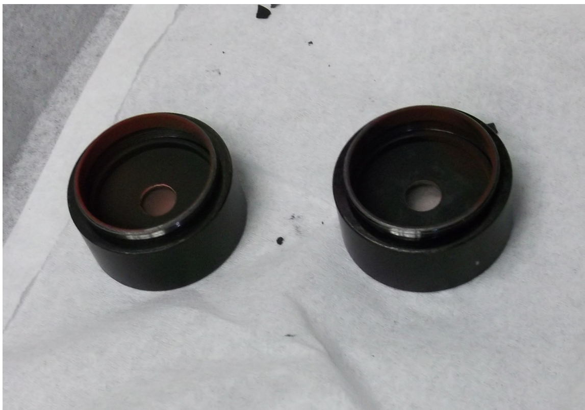
Figure 2.6: Cell windows and baffles are mounted into lens tubes for easy cleaning and modification. Pink residue is a thin layer of Nile Red.
