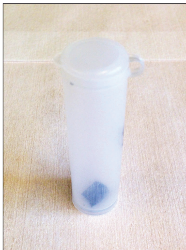
Figure A.6: Plastic vial for growth wafer sonication. The vial is just big enough to fit a piece of the growth wafer so that only a small amount of methanol is needed to submerge the substrate.
