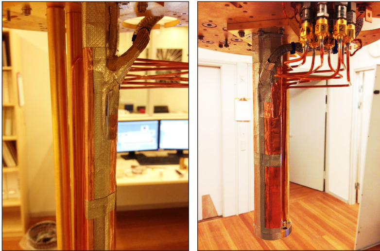
Figure B.4: New coldfinger of Triton 1, modified by wrapping sheet copper around the coldfinger struts to contain the DC looms traveling between the sample puck and the rest of the mixing chamber plate.
