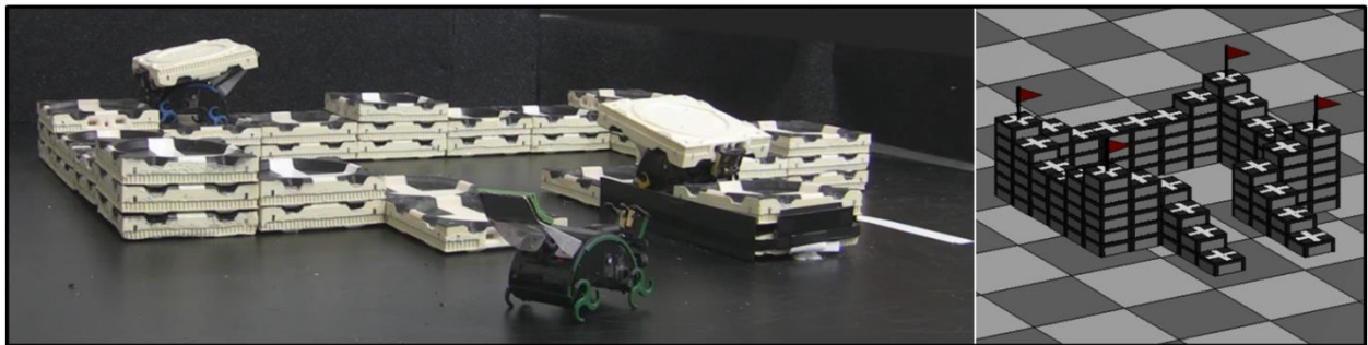
Figure 1.3.a. Collective construction of a castle-shaped structure, left: with real robots, right: in simulation.
