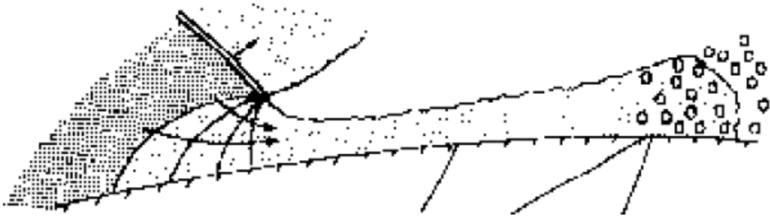
Figure 1.3: Detachment of a shockwave in the liquid from the solid surface, and consequent ejection of the splash at the base of the drop. From Lesser and Field (1983). Courtesy Annual Reviews Inc.
