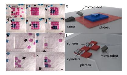
Figure 4. Three-dimensional micro-robotic coding of material composition
