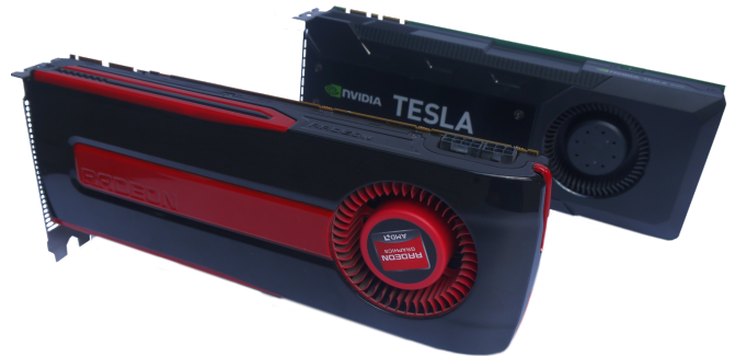
Figure 5. AMD Radeon HD 7970 and a Nvidia Tesla K20 GPU cards used for the numerical tests.
