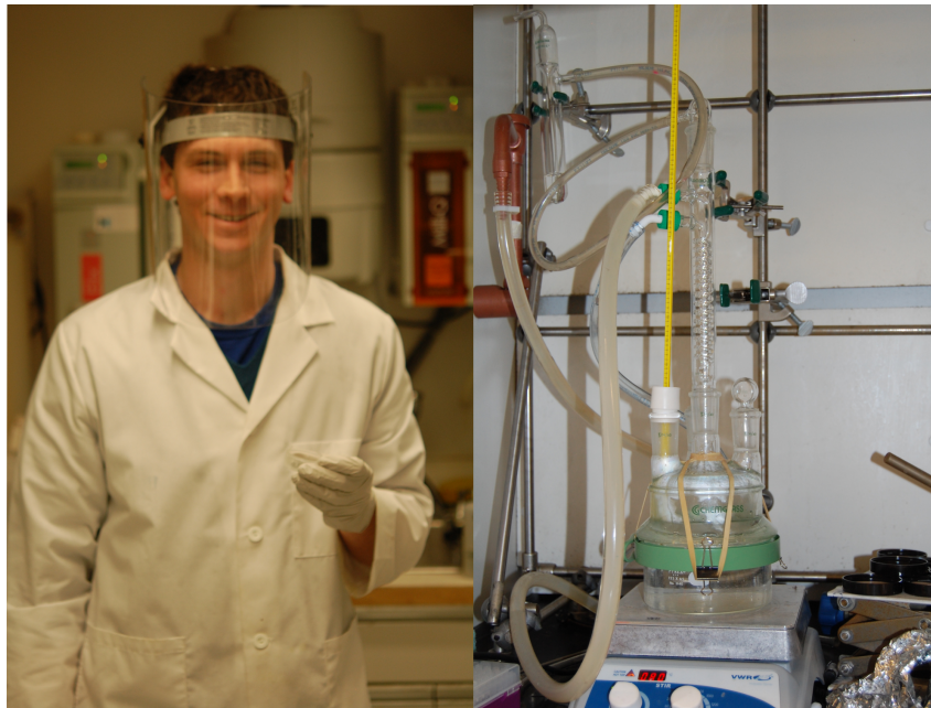
Figure B.2: Left: experimentalist wearing a facemask after etching wafer. Right: Hot KOH wafer etching set-up.
