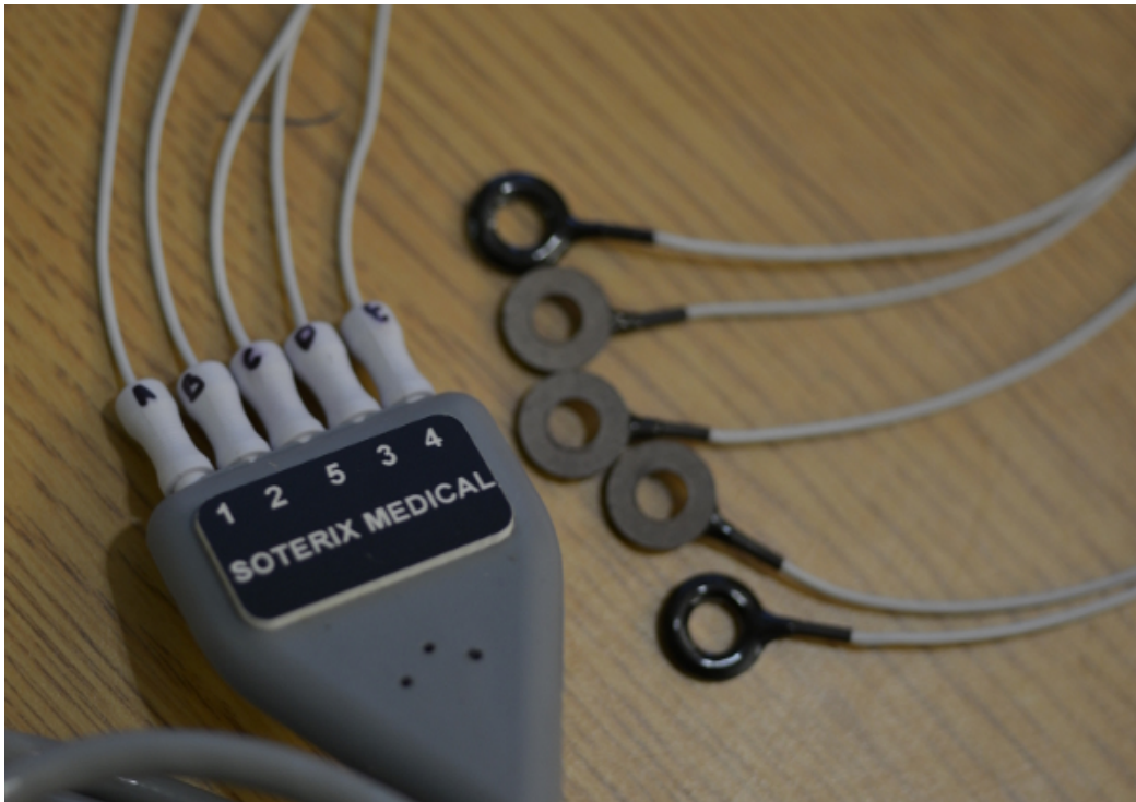
Figure 2. Ag/AgCl sintered ring electrodes, with smooth rounded (black) and rough surfaces. Electrodes are connected to the matching receivers on the 4x1 adapter output cable.
