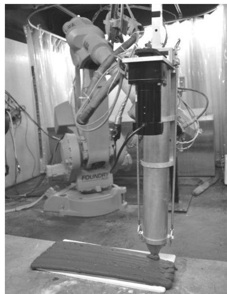
Fig. 7 Ceramic deposition in progress
