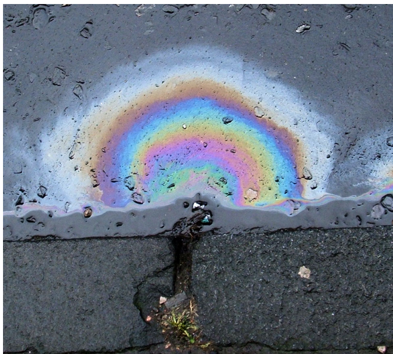
FIGURE 2.1: Photograph of an diesel film of varying thickness on water demonstrating thin film interference. From ref. [3]
