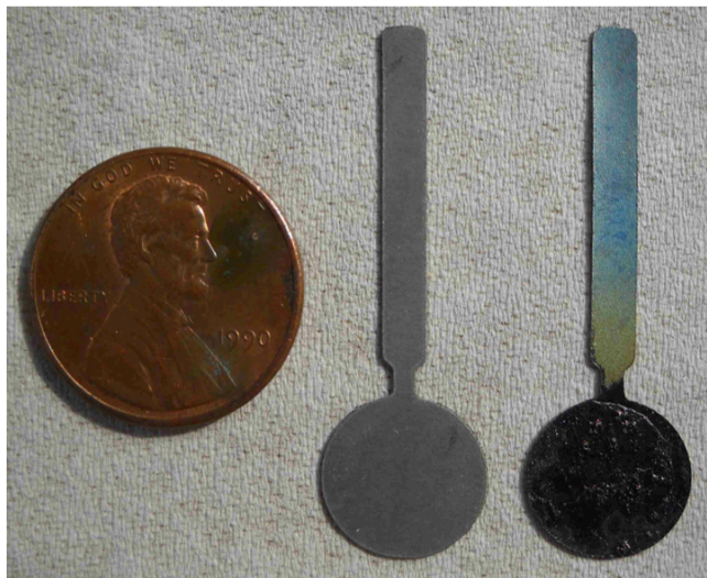
Figure 3.1. Image of both an RuO 2 -coated and uncoated niobium tab electrode. A U.S. penny is also shown for scale.
