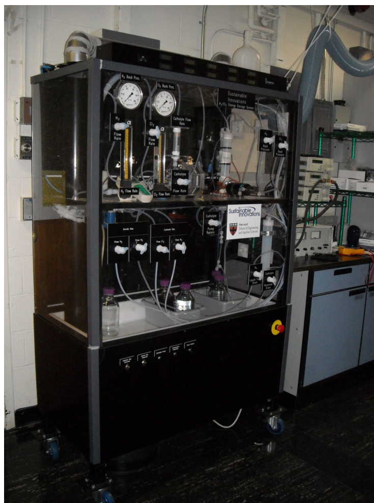
Figure 2.3. Image of the test bench designed by Sustainable Innovations. The entire cavity of the bench is held under negative pressure for safety reasons.
