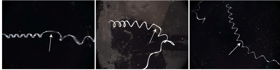
Figure 3.2.1: The same fiber ribbon is progressively cut lengthwise to yield narrower and narrower strips. Arrows indicate helical perversion in all panels. Left: The intact fiber ribbon. Middle: Resulting fiber ribbon from one lengthwise cut. Right: The fiber ribbon from the middle panel is cut lengthwise again, yielding an even narrower ribbon with the same shape.
